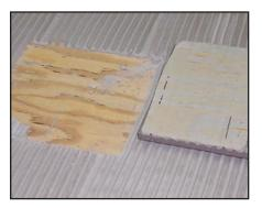
Competing polymer-modified products vary in performance, sometimes providing weak bonds to difficult substrates, such as plywood.
